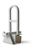
Some grab bars can be mounted on the edge of the bath tub by a clamping mechanism. The turning knob located on the outside of the clamping mechanism is used to secure the grab bar. The key feature of this grab bar is that it is made of plastic and stainless steel. (Note: Do not use with fiberglass bathtubs because it can damage the fiber- glass).
