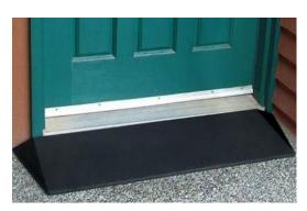
Threshold ramps can prevent stumbling and also provide accessibility to the users of a wheelchair or scooter. Rubber threshold ramps have advantages over metallic or wooden ramps in terms of traction, and shock absorption. It can be trimmed to custom fit various door- ways. It is available in various sizes. (Note: Threshold ramps may be needed for both sides of a threshold)
