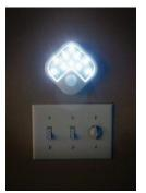
Using automatic LED lights is an efficient way to illuminate dark hallways to prevent falls. The motion sensors activate the light whenever movement is detected, and the auto shut-off feature turns the light off when there is no movement for a preset duration of time.
